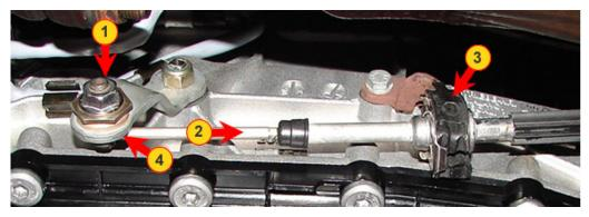
Always check the shifter cable bracket **3** to make sure it was not bent during transmission removal.
