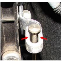
The cable should not touch the lever at any time, even if the lever is moved back and forth. If the cable does come in contact then check for a bent lever or a bent cable bracket.
